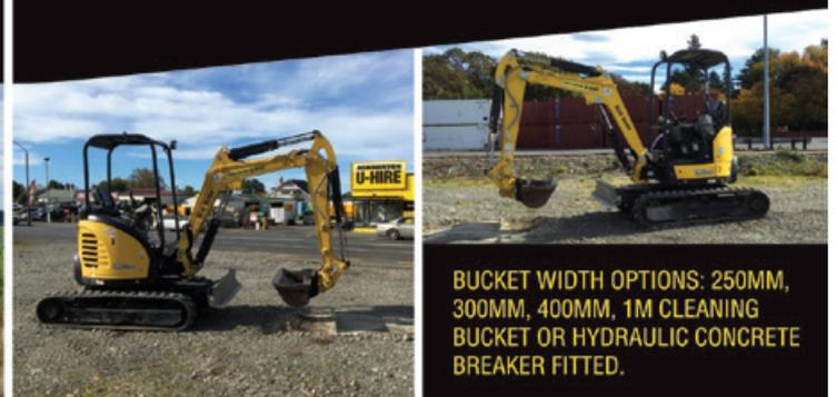
BUCKET WIDTH OPTIONS: 250MM, 300MM, 400MM, 1M CLEANING BUCKET OR HYDRAULIC CONCRETE BREAKER FITTED.
